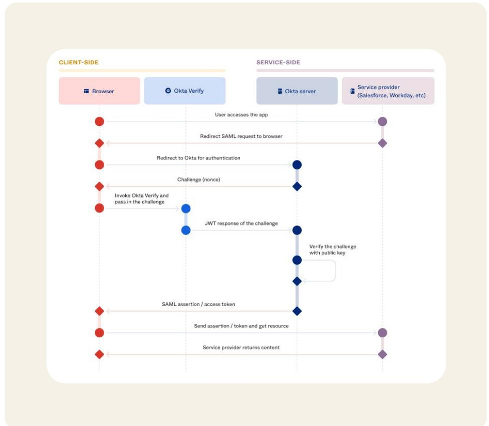
A typical SAML SSO flow, with FastPass
