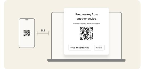
A WebSocket tunnel is established between the two devices, and a cryptographic handshake establishes a secure, authenticated connection.
